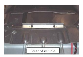
• Place floor in vehicle and butt up to rear-mounting foot.
